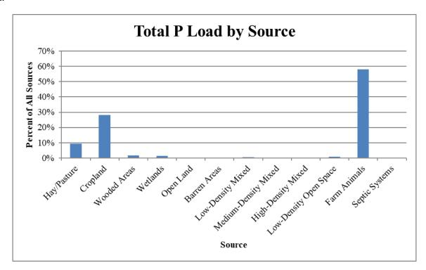
Figure 7: Total Phosphorus Load by Source in the French Stream Watershed
